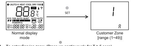
4 To enter Service zone: (Press set continuously for  $T \ge 5$  secs)
