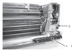
Disconnect CN-STM1, CN-STM2 and CN-STM3 from electronic controller.
