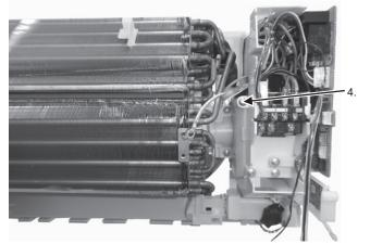
Remove 1 screw from control board complete. Then pull out the control board complete.
