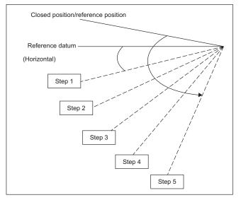
\* The horizontal vane angle tolerance is within +/- 5 degree.
