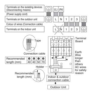
Secure the connection cable onto the control board with the holder. 6
