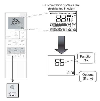
2 Cannot enter this customization mode under the following conditions:  $\widehat{1}$  Operation ON.
